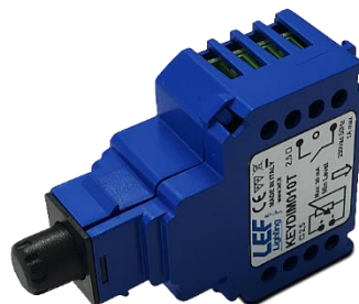
(LEF) KEYDIM010T Passive Analogic 0-10V controller
